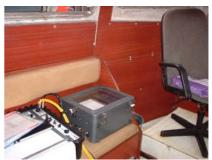
Odom Hydrotrac Echosounder onboard survey
