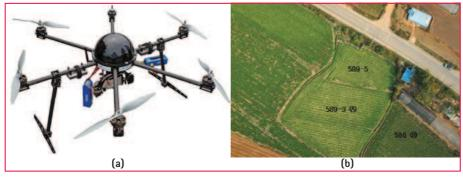
Figure 2: LX-UAV (Hexacopter) (a), and UAV digital image (b)
